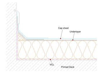
At all skirtings and upstands, the waterproofing should be at least 150mm <u>above</u> the level of the finished roof. Care must be undertaken not to bridge over any DPC or Cavity Tray positions.
