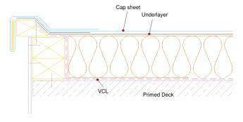
Check kerbs should be constructed to form a 50mm water check to prevent water from running over the edge incorporating a welted drip detail. In warm roof build ups a timber hard edge should be incorporated.
