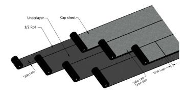
Figure 1 Setting Out to Staggered Laps
